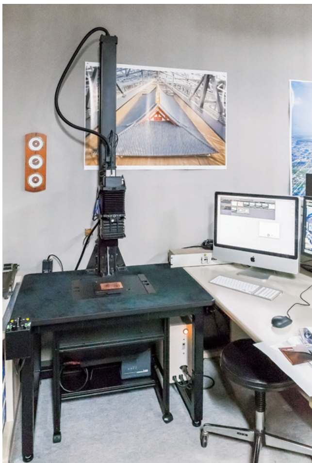
複写式高精細写真デジタル化装置 Digital high-definition photo duplicating device
