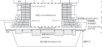
Fig. 76: Schematic diagram of the lower platform reassembly work
