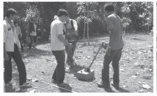
Fig 5.Geopenatrating Rader Survey
