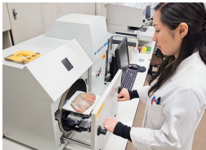
保存修復科学：建造物の彩色調査 Investigation of paintings on traditional building
